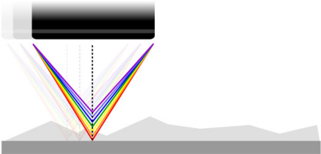
Nanovea optical pens have zero influence from sample reflectivity. Variations require no sample preparation and have advanced ability to measure high surface angles. Capable of large Z measurement ranges. Measure any material: transparent/opaque, specular/diffusive, polished/rough. Measurement includes: Profile Dimension, Roughness Finish Texture, Shape Form Topography, Flatness Warpage Planarity, Volume Area, Step-Height Depth Thickness and many others.
