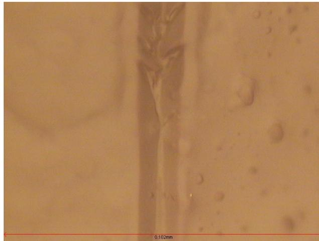
Figure 8 : Micrograph of the Initial Cracking – Aluminium
