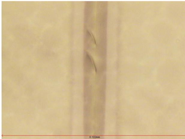
Figure 2 : Micrograph of the Initial Cracking – Glass
