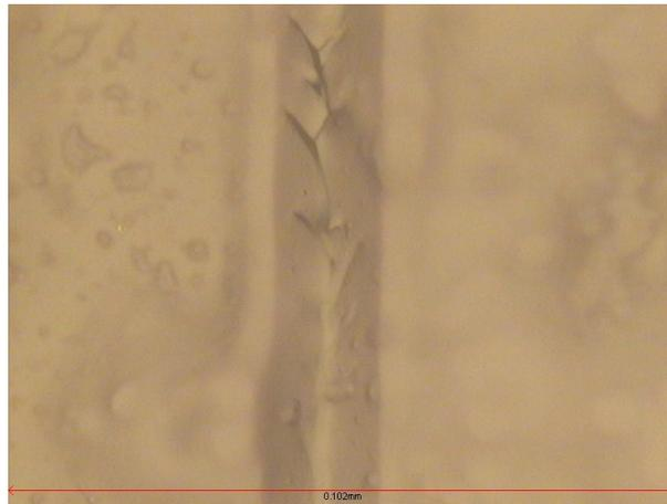
Figure 5 : Micrograph of the Initial Cracking – Plastic
