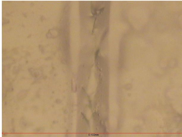
Figure 6 : Micrograph of Continuous Cracking – Plastic
