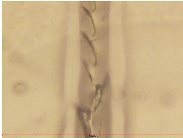
Figure 3 : Micrograph of Continuous Cracking – Glass
